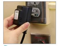
Plug the Classic-Check control unit's power supply cord into the electrical outlet.
