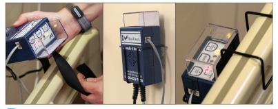
To secure the Classic-Check control unit out of the reach of the individual, attach the control unit to the bed frame\* using the standard Velcro® strap, or to the headboard using an optional wire holster.
