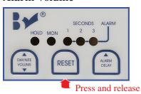
The alarm volume can be adjusted separately for both the DAY and NITE modes. First set the mode for which you are changing the volume (see other side). Press *and hold* the RESET button, then press and hold the DAY/NITE VOLUME button. Release the RESET button to hear current setting. Then press and release the RESET button until desired volume is obtained. Release all. Press/release RESET once more to lock the setting.
