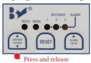
Press and release DAY/NITE button to switch between DAY and NITE modes. NITE mode is indicated by a blue light in the splash guard.
