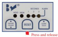
Press and release the RESET button to go from MONITOR to HOLD, or from HOLD to MONITOR, or to silence an alarm. Please note that if the system is on HOLD, it will reset itself and resume monitoring if weight is placed on the Sensormat<sup>®</sup>. In addition, if the RESET button is pressed to put on HOLD and weight remains on the Sensormat<sup>®</sup>, the unit will return to monitoring mode in 25 seconds.
