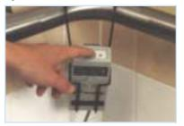
**G.** To remove the patient/resident from the toilet seat, press the RESET button on the Chair-Check II one time. This puts the Chair-Check II into standby mode.
