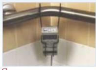
**C.** Using a Chair-Check wire holster, attach the Chair-Check II to a bathroom handrail where readily accessible to the caregiver, and out of reach of the patient. Record date put in use on Sensormat cord tag.
