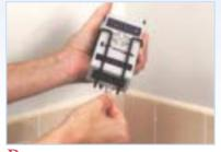
**B.** Plug the Potty-Check Sensormat's phone-style jack into the Chair-Check II control unit. Delay should be set at 0 or 1 second (see User Guide).
