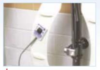
A. Remove Sensormat<sup>®</sup> from plastic container. Use the adhesive backing on the Sensormat to properly position it. It is usually placed between the two seat bumpers, but may be placed on the top edge of the toilet bowl. Locate it forward for lighter patients and rearward for heavier patients.
