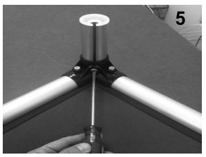
5) Insert legs into bottom corner. Rotate leg so slot aligns with set screw hole. Secure in place with set screw. This is purposely a tight fit so it will take some effort to fully tighten screws. 6) Turn bed over and fully tighten all screws and nuts.
