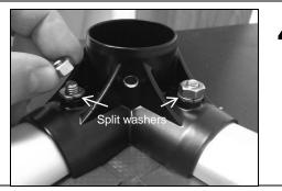
4) Place a bottom corner bracket over pipes, insert screws through openings, place split washer over screw, secure with a nut and hand tighten. Insert and secure second screw. Repeat process at each of other three corners.
