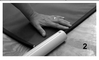
2) Insert fabric sleeves into the channel on each length of pipe.
