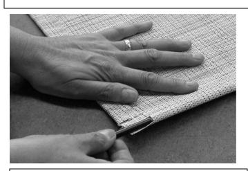
1) Lay fabric flat with underside facing up and insert cording into sleeve. Note that 40oz Vinyl fabric comes with cording in the sleeve.
