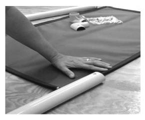
For each nest, insert the fabric into the channel on each length of frame pipe. There are 2 long sides and 2 short sides for each nest.
