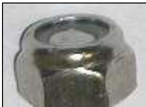
Figure 1. Correctly tightened. Screw is flush with nylon locking material
